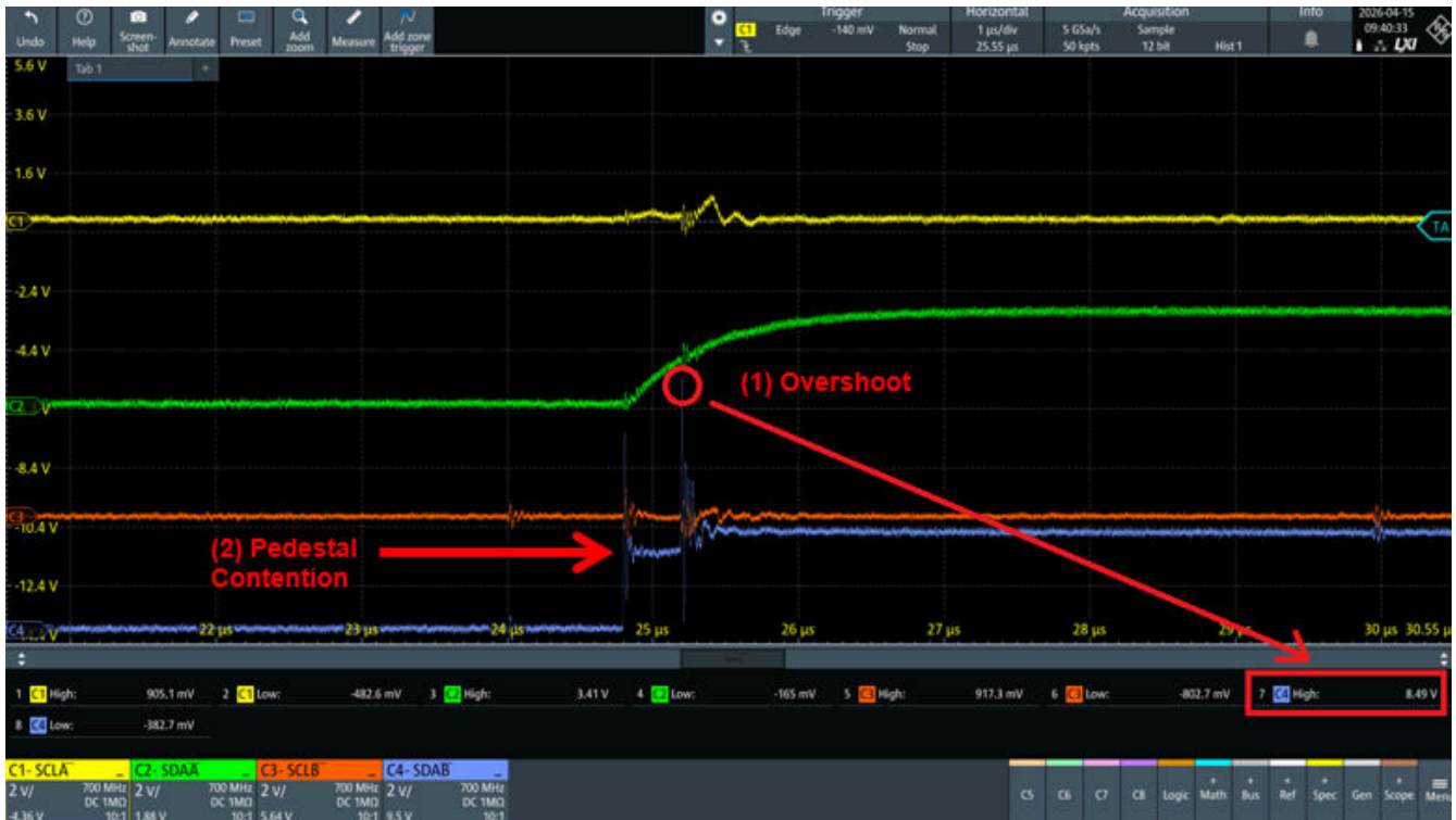
Figure 2-2. Overshoot Spike Test from ICT
