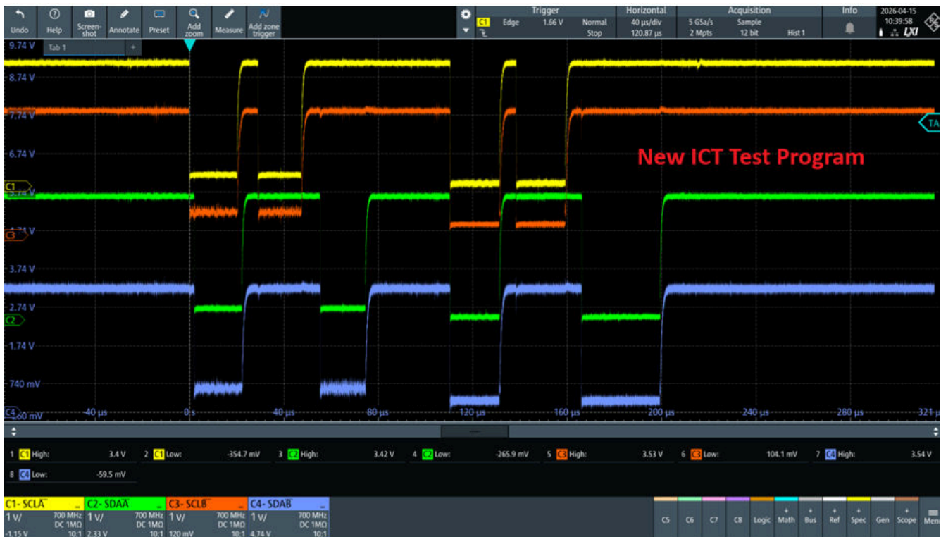
Figure 2-4. New ICT Setup with Software and Hardware Changes Reduces Overshoot/Undershoot Behavior and Resolves B-side Pedestal Contention
