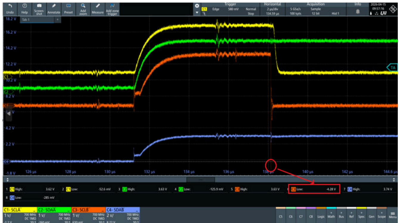
Figure 2-3. Undershoot Spike Test from ICT
