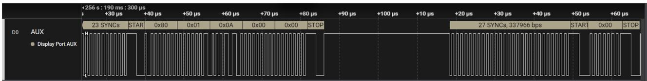
Figure 4-5. Logic 2 AUX Waveform Utilizing AUX Analyzer Extension
