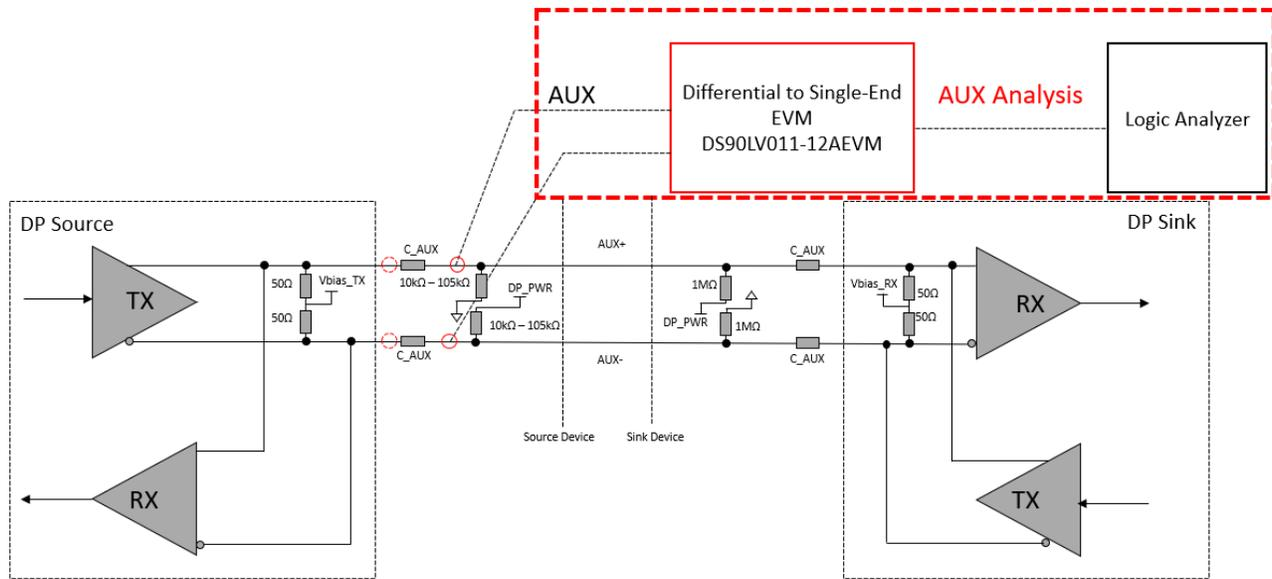
Figure 4-1. Block Diagram Integrating DS90LV011-12AEVM
