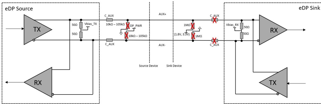
**Figure 3-2. eDP AUX CH Differential Pair**
