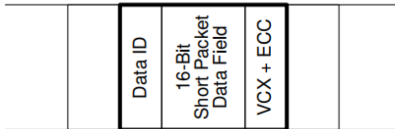
Figure 3-2. MIPI CSI-2 Short Packets
