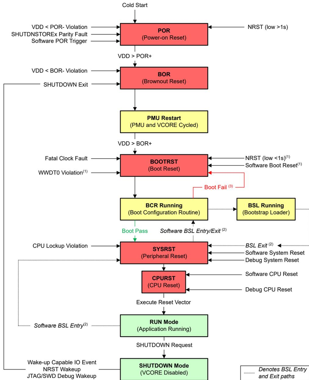
Figure 3-1. AM13E230x Reset Levels
