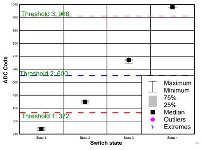
Figure 9. Switch State Verification Across Temperature
