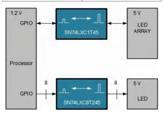
Figure 1. Processor Driving LED Example
