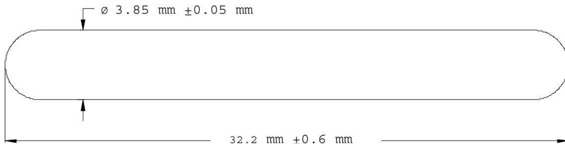
**Figure 1. Dimensions of the TI 32 mm Transponder**
