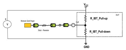
**Step 2:** Measure the voltage with a multimeter (V-Center) at the input pin of the register to be measured for IBT value. Measure after the R-stub on the module, and close the register if possible with respect to the ground on the memory module.
