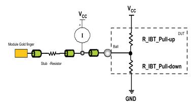
**Result 3:** R\_IBT\_Pull-down value can be calculated using Ohm's Law as the VDD value is known from Step 1. Also, the current flowing through R\_IBT\_Pull-down IBT resistance is known, having been measured from Step 4.
