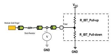
**Result 1:** The measured voltage V-Center must be equal to VDD/2 within the valid tolerance of the specification. Any deviation of this voltage from VDD/2 gives the mismatch between the R\_IBT\_Pull-up and the R\_IBT\_Pull-down resistance of the IBT.
