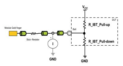
**Result 2:** The R\_IBT\_Pull-up value can be calculated from Ohm's Law as the VDD value is known from Step 1. Also, the current flowing through R\_IBT\_Pull-up IBT resistance is known, having been measured from Step 3.
