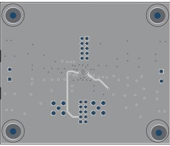
Figure 6. Bottom Layer Routing
