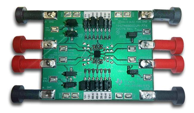
This user's guide describes the operational use of the TPS7A8801EVM-776 evaluation module (EVM) as a reference design for engineering demonstration and evaluation of the TPS7A8801RTJ, low-dropout linear regulator (LDO). Included in this user's guide are setup and operating instructions, thermal and layout guidelines, a printed circuit board (PCB) layout, a schematic diagram, and a bill of materials (BOM).
