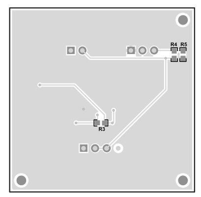
Figure 2. Bottom Layer Routing
