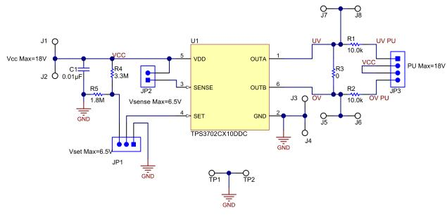
Figure 3. TPS3702CX33EVM-683 Schematic
