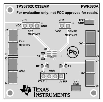
Figure 1. Top Layer Routing
