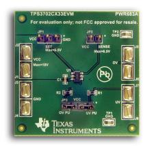
This user's guide describes the operational use of the TPS3702CX33EVM-683 evaluation module (EVM) as a reference design for engineering demonstration and evaluation of the TPS3702CX33, an ultralow-power, wide supply voltage, window voltage detector for over and undervoltage monitoring. Included in this user's guide are setup instructions, a schematic diagram, printed circuit board (PCB) layout drawings, and a bill of materials for the EVM.
