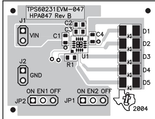
Figure 3. Top Layer Routing
