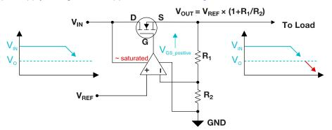
Figure 1-2. Dropout Limitation of NMOS LDO
