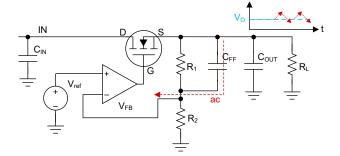
Figure 2-1. Open Loop Small-Signal Model of NMOS LDO
