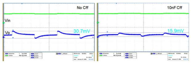
Figure 3-3. Load Transient Performance Comparison
