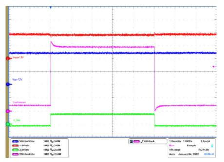
Figure 3-4. Transient Response of Modified Vout=1.2 V (with 10 nF C<sub>ff</sub>)
