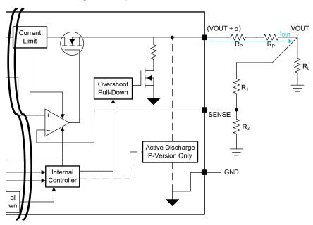
Figure 2-3. IR Drop Compensation by Remote\_Sense with Resistor Network
