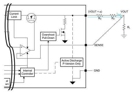
Figure 2-2. IR Drop Compensation by Remote\_Sense
