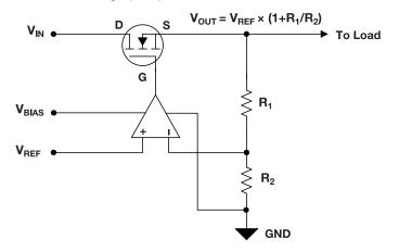
Figure 1-3. NMOS LDO with an External Biasing
