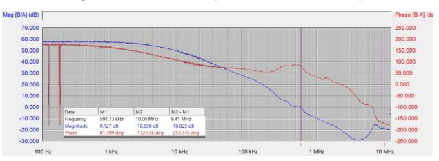
Figure 3-1. Simulated Bode Plot (Vin=1.8 V, Vo=1.2 V, lout=100 mA)
