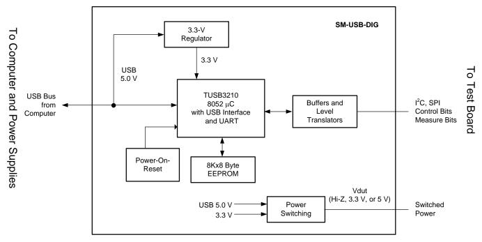
Figure 4. USB DIG Platform Block Diagram
