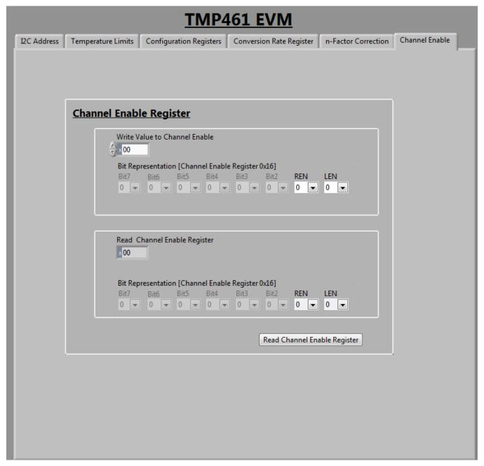
Figure 18. TMP461-SP Channel Enable Register Tab
