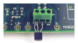
Figure 8. Remote NPN Setup
