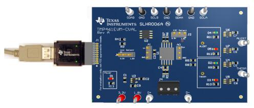
Figure 5. Connecting the SM-USB-DIG Platform
