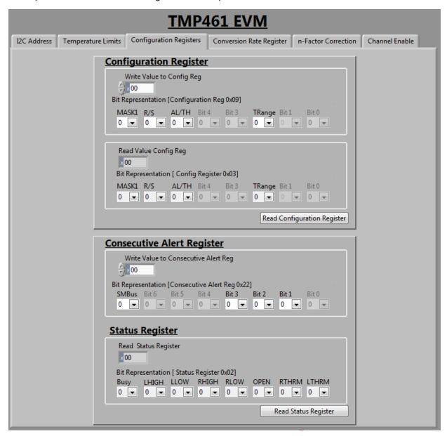
Figure 17. TMP461-SP Configuration Registers Tab
