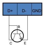
Figure 7. Connection for the NPN Transistor to J4
