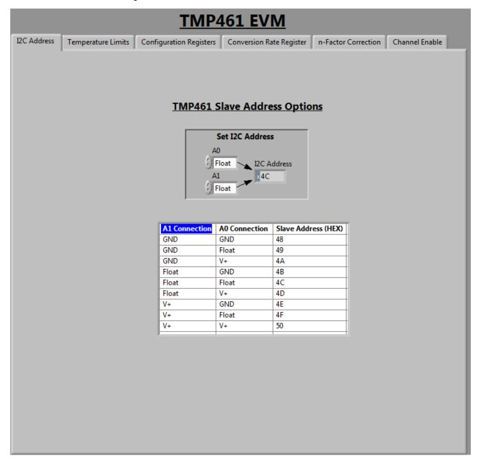
Figure 15. I2C Address Tab
