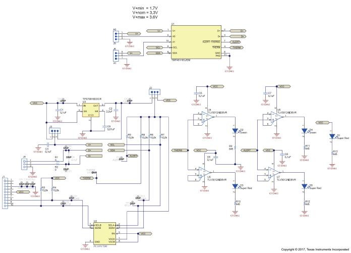
Figure 20. TMP461EVM-CVAL Board Schematic
