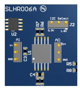
Figure 9. Slave Address Connections (A0, A1)
