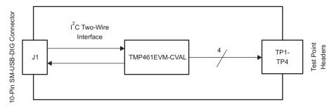
Figure 3. TMP461EVM-CVAL Test Board Block Diagram
