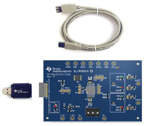
Figure 1. Hardware Included With TMP461EVM-CVAL Kit
