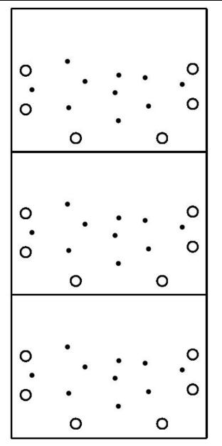
Figure 6. INA199EVM Bottom Solder Mask
