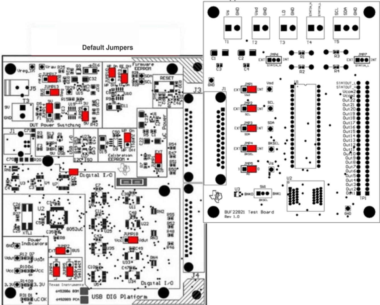
Table 4 summarizes the function of the BUF22821 Test Board jumpers. For most application, jumpers 2 through 5 are all set to the default positions.
