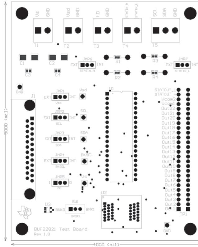
Figure 28. BUF22821EVM-USB PCB Top Layer (Component Layout)
