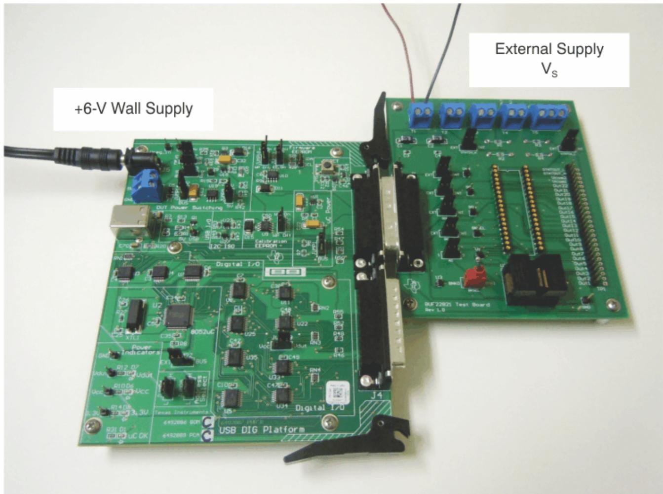
**Figure 6. Connecting External Power to the BUF22821EVM-USB**
