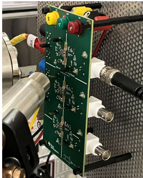
Figure 5-11. Device Under Test Lined Up With the Beam
