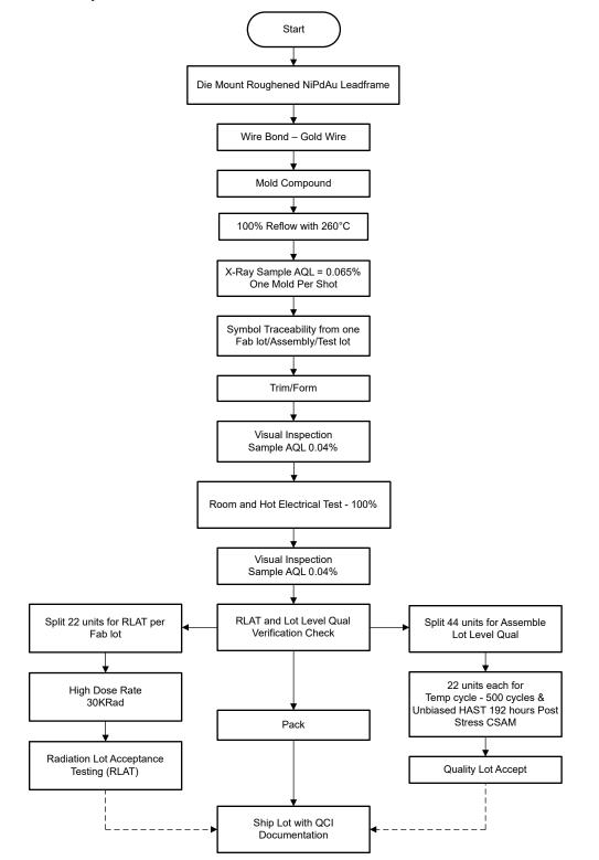
Figure 4-1. OPA4H199-SEP Space Enhanced Plastic Production Flow Chart
