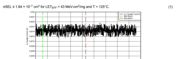
Figure 5-1. Current vs Time (I vs t) Data for Vs Current During SEL Run # 32
