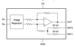
Figure 2-1. Functional Block Diagram of the INA240-SEP
