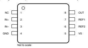
Figure 3-1. INA240-SEP Pinout Diagram
