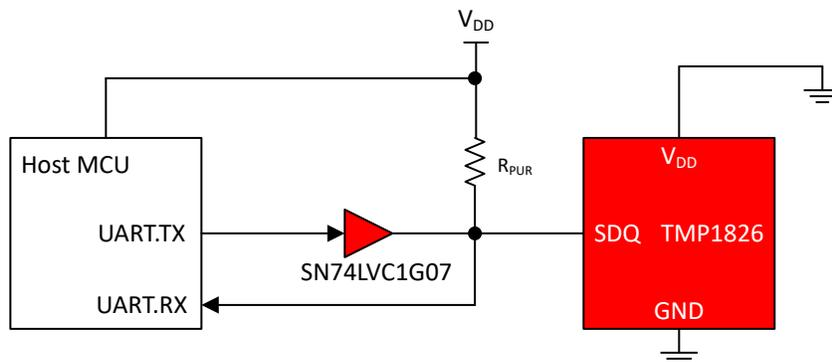
Figure 2-6. UART Interface for TMP1826
