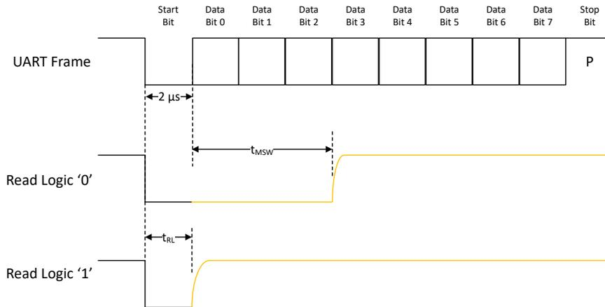
**Figure 2-10. UART Frame Overlay for Overdrive Read**
