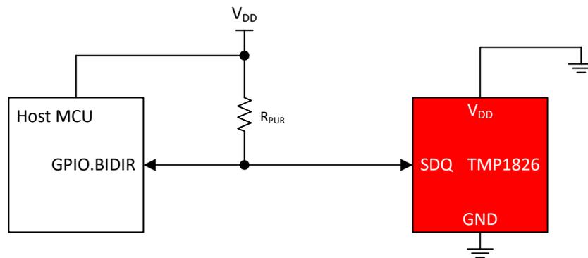
**Figure 2-1. Bidirectional GPIO Interface for TMP1826**
