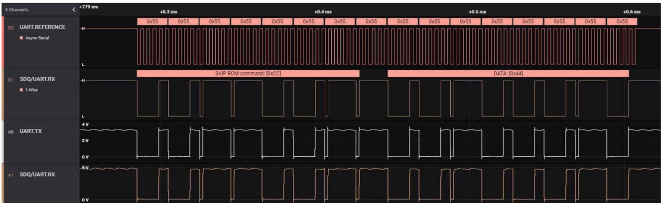
Figure 2-12. Scope Capture of Write Transfer
