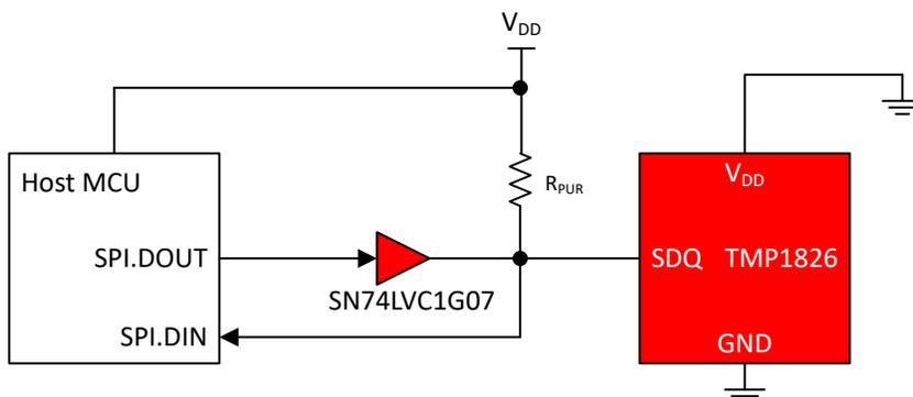
Figure 2-14. SPI for TMP1826
