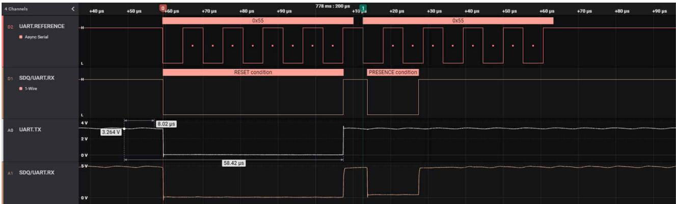
Figure 2-11. Scope Capture of Bus Reset and Response
