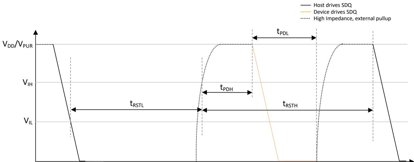
Figure 1-2. Bus Reset and Response
