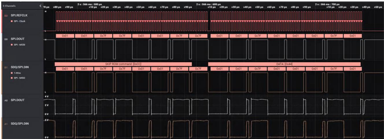
Figure 2-16. Scope Capture of Write Transfer
