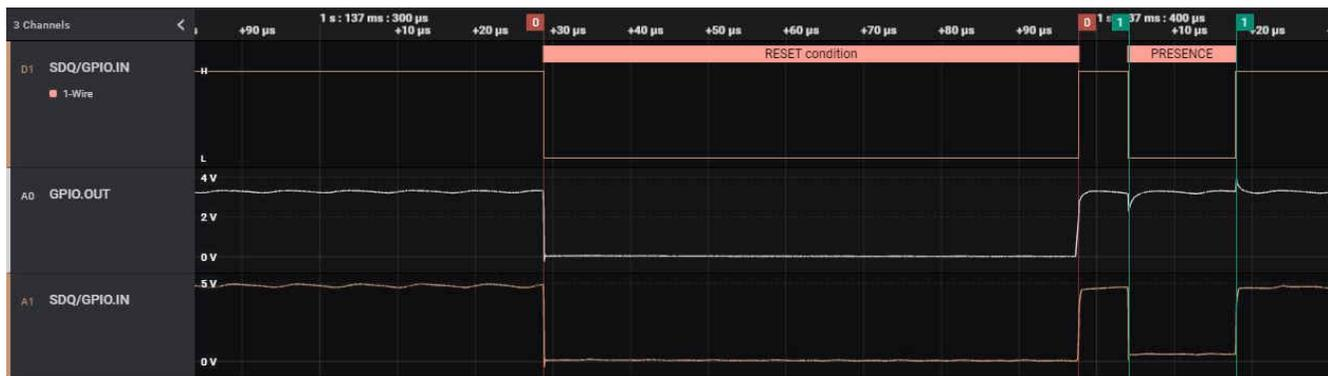
Figure 2-3. Scope Capture of Bus Reset and Response
