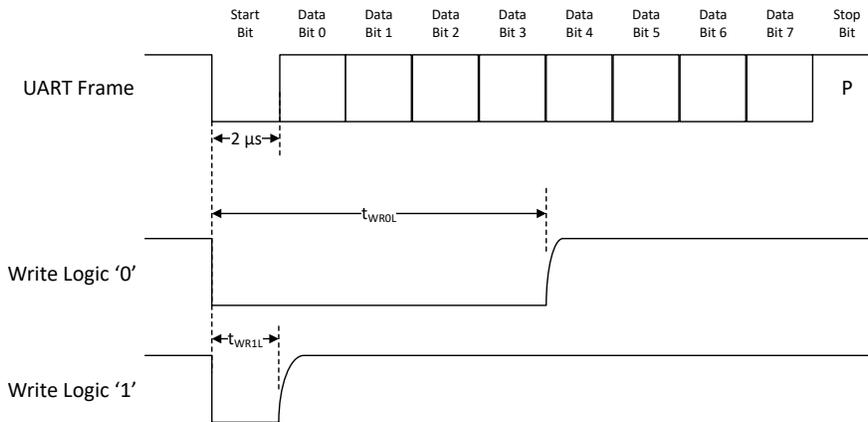
**Figure 2-9. UART Frame Overlay for Overdrive Write**
