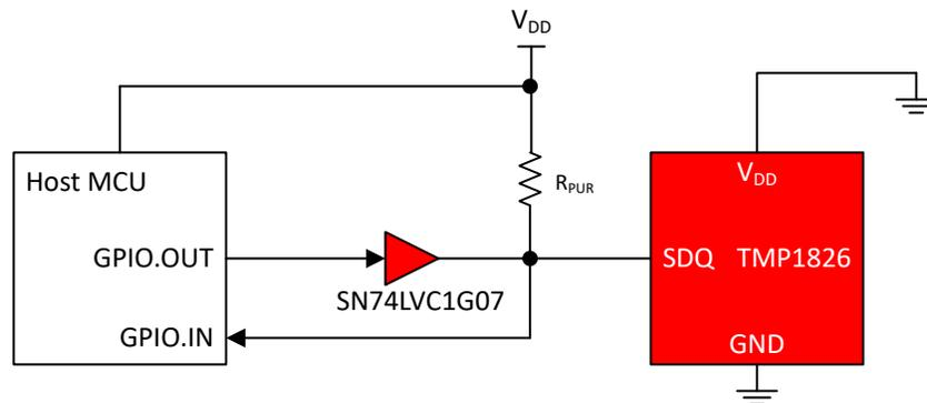
**Figure 2-2. Push-Pull GPIO Interface for TMP1826**
