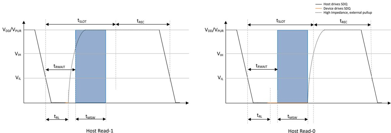
Figure 1-4. Host Read, Device Write
