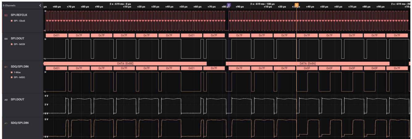
**Figure 2-17. Scope Capture of Read Transfer**
