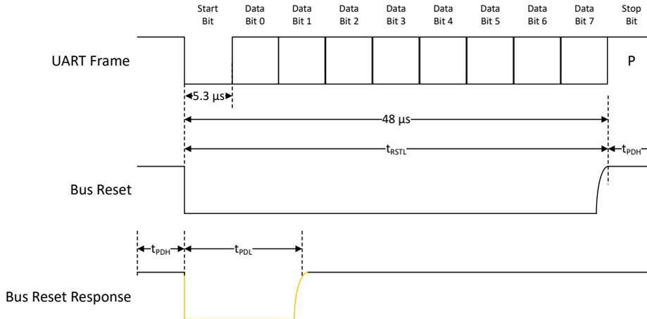
**Figure 2-8. UART Frame Overlay for Overdrive Bus Reset and Response**
