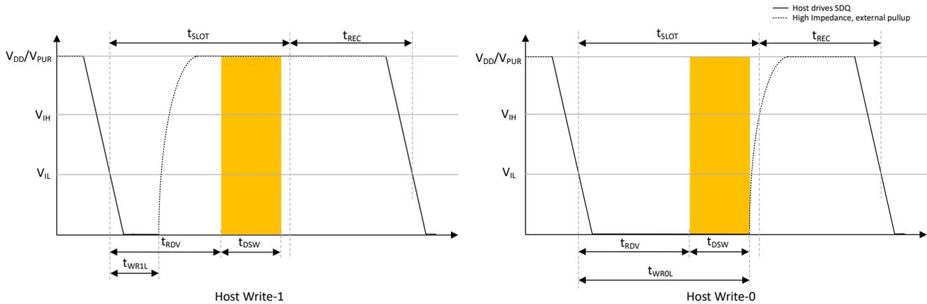
Figure 1-3. Host Write, Device Read
