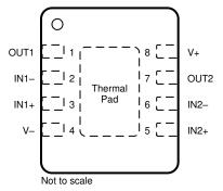
Figure 3. Pin Diagram (WSON-8 Package)
