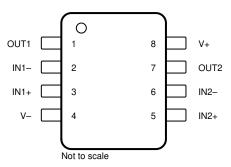
Figure 2. Pin Diagram for TSSOP-8, VSSOP-8, SOIC-8, and SOT23-8 packages
