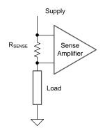
Figure 1. High-Side Current Sensor
