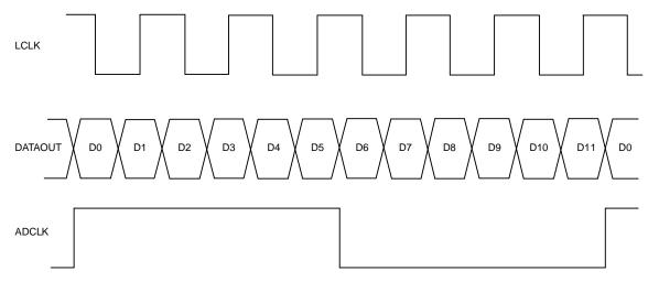
Figure 1. Timing and Alignment of ADS527x Data with LCLK and ADCLK
