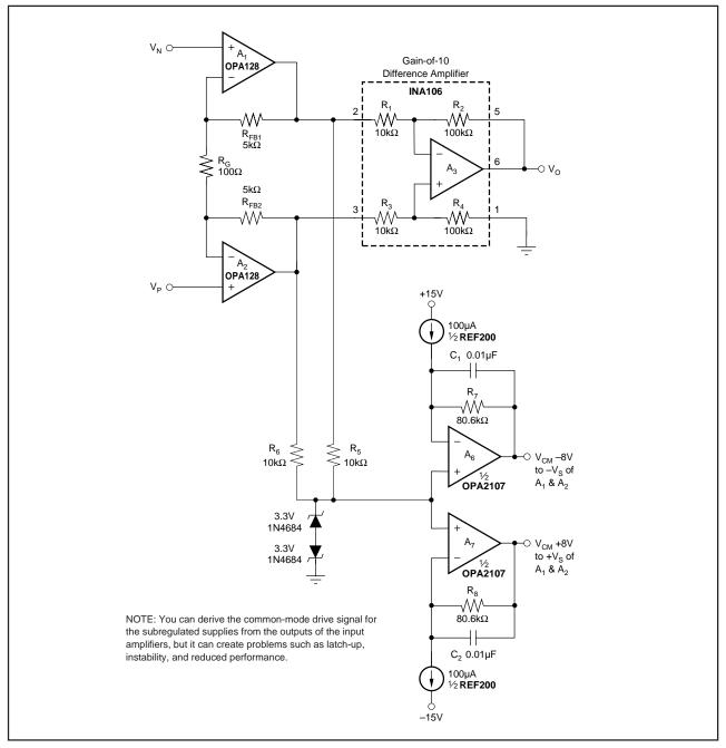
FIGURE 6. Boosted Electrometer Instrumentation Amplifier.
