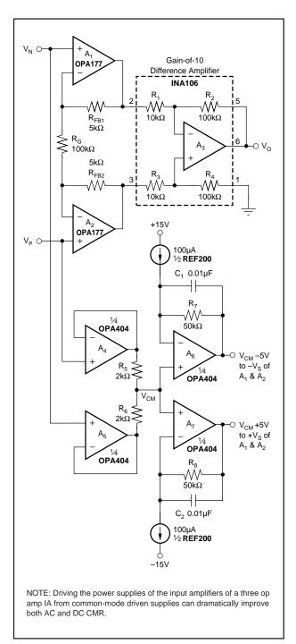
FIGURE 2. Boosted Instrumentation Amplifier.
