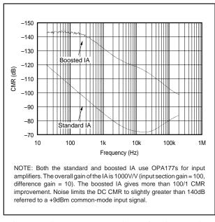
FIGURE 5. CMR vs Frequency Comparison between Standard Three Op Amp IA and Boosted IA.
