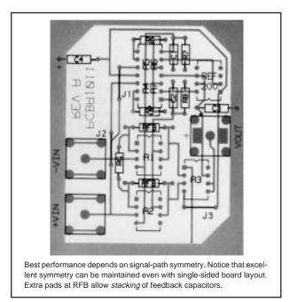
FIGURE 8. Printed Circuit Layout of Figure 2 Boosted IA.
