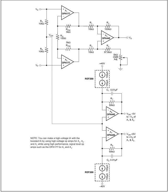
FIGURE 4. High Voltage Instrumentation Amplifier.
