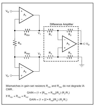
FIGURE 1A. The Three Op-Amp Instrumentation Amplifier.
