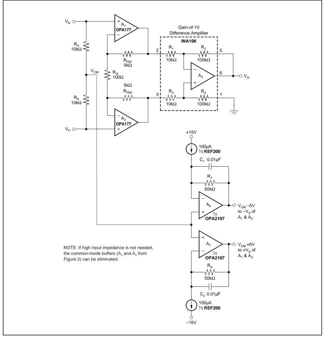
FIGURE 3. Simplified Boosted Instrumentation Amplifier.
