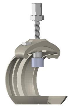
Figure 2-8. Magnet and Handle Assembly
