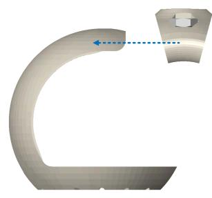
Figure 2-5. Connecting the Slider
