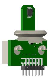
Figure 2-10. Clip With Attached EVM
