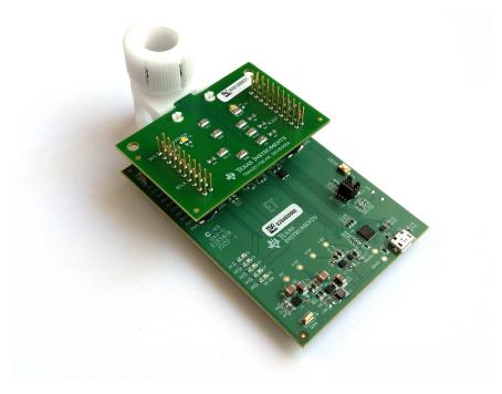
Figure 9. Rotate & Push Module on EVM
