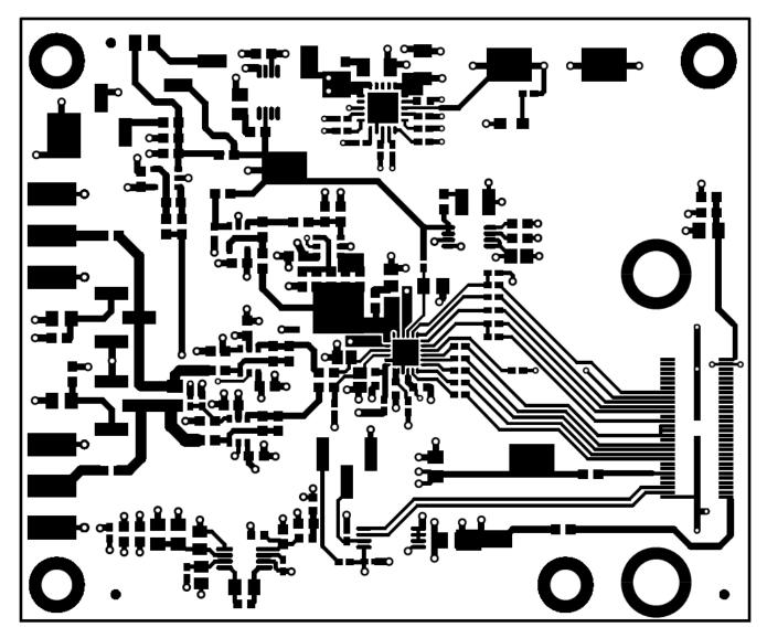
Figure 16. ADS8910BEVM PCB Layer 1: Top Layer
