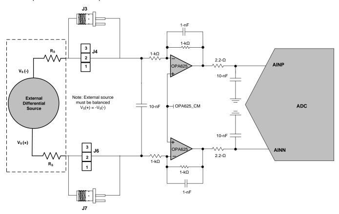
Figure 1. OPA625 Differential Input Driving Path
