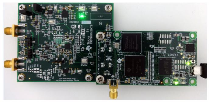
Figure 7. EVM-PDK Hardware Setup and LED Indicators
