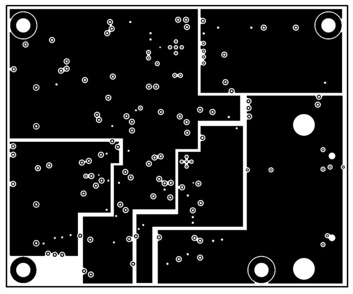
Figure 18. ADS8910BEVM PCB Layer 3: Power Planes
