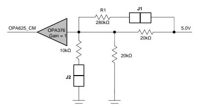
Figure 2. Common-Mode Selection Jumpers
