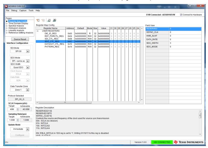
Figure 9. EVM GUI Global Input Parameters
