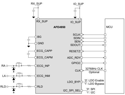
Figure 3. Reference Schematic of an ECG Acquisition System Using AFE4950
