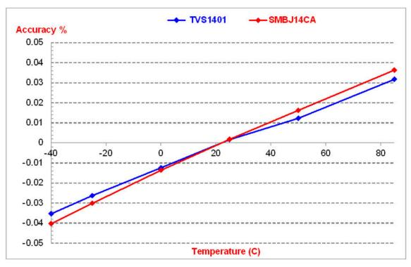
RTD Measurement Accuracy at RTD =  $100 \Omega (0^{\circ}C)$
