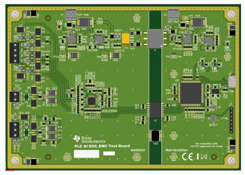
ADS124S08 Test Board With Input Protection Circuity
