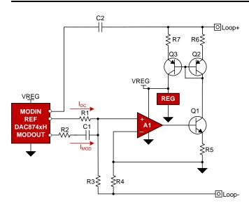
Figure 2. Loop-Powered FF/PA Transmitter Circuit (V-to-I Converter)
