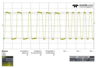
Figure 3. Bus Voltage with FF/PA Signal Transmitted
