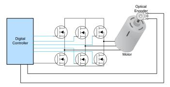
Figure 3. Digital Control loop for motor
