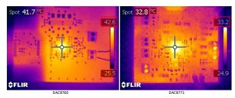
Figure 3. Thermal Comparison of DAC8760 and DAC8771 with Adaptive Power Management
