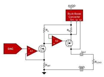
Figure 2. 3-Wire Transmitter With Adaptive Power Management
