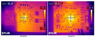
Figure 4. Thermal Comparison of DAC8760 and DAC8771 With Adaptive Power Management
