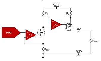
Figure 1. 3-Wire Current Transmitter Circuit
