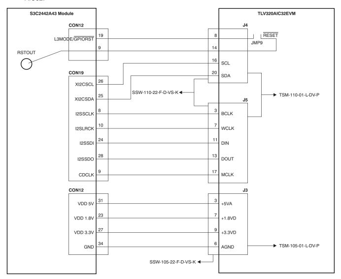
Figure 2. TLV320AIC32EVM Connections to Samsung SMDK2440X Module
