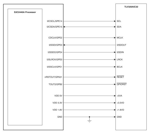
Figure 1. TLV320AlC32 Connections to Samsung SC32440A Processor
