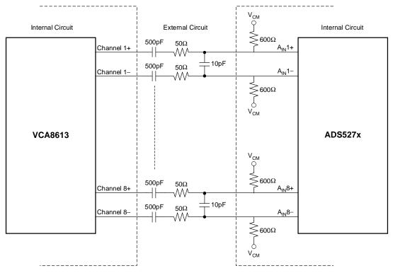
Figure 3. AC-Coupled Interface Between VCA8613 and ADS527x
