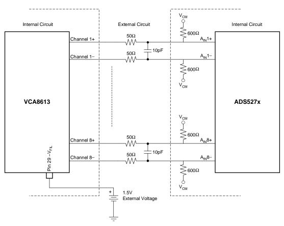
Figure 4. DC-Coupled Interface Between VCA8613 and ADS527x
