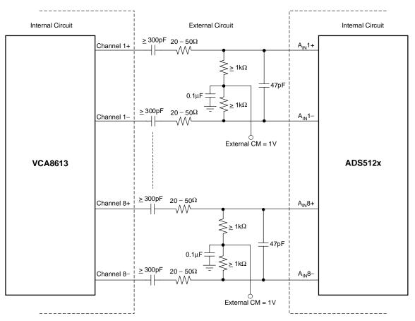
Figure 2. AC-Coupled Interface Between VCA8613 and ADS512x
