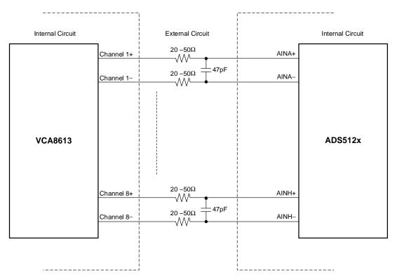
Figure 1. DC-Coupled Interface BetweenVCA8613 and ADS512x
