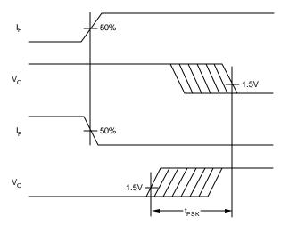
Figure 15. Illustration of the Propagation Delay Skew—t<sub>PSK</sub>
