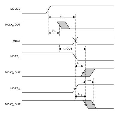
Figure 10. Delay Time on the Rising Edge of MCLK
