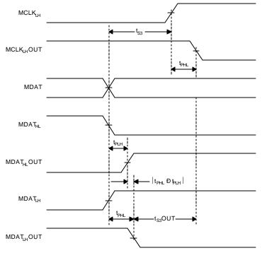
Figure 8. Setup Time on the Rising Edge of MCLK
