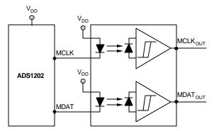
Figure 1. Reference Signals for the ADS1202 and the Optocoupler
