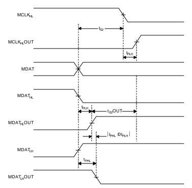
Figure 7. Setup Time on the Falling Edge of MCLK
