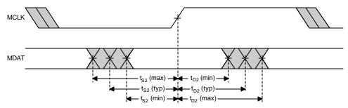
Figure 3. The ADS1202 MDAT Output Signal on the Rising Edge of MCLK
