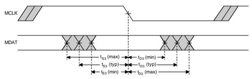
Figure 4. The ADS1202 MDAT Output Signal on the Falling Edge of MCLK
