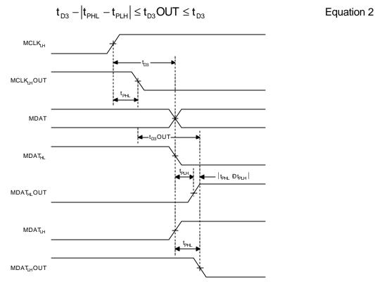
Figure 6. Delay Time on the Rising Edge of MCLK
