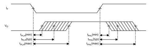
Figure 13. Propagation Delay Time of Low and High Output Levels
