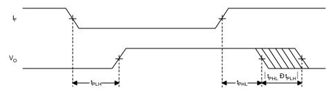
Figure 14. Pulse-Width Distortion of the Output
