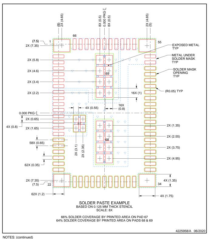
6. Laser cutting apertures with trapezoidal walls and rounded corners may offer better paste release. IPC-7525 may have alternate design recommendations.
