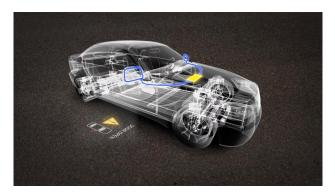
Figure 2. Vehicle infrastructure routing to connect the DGP module to the central ECU.
