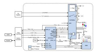
*Figure 7.* Typical system block diagram for a basic mobile projector.
