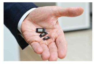
*Figure 8.* Three different sizes of DLP Pico DMDs – the smallest has a micromirror array diagonal of 0.2 inches.
