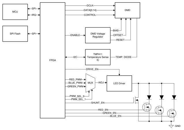
Figure 1. Dynamic Ground Projection Electronics Block Diagram
