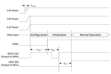
Figure 3. Power-up Timing Diagram
