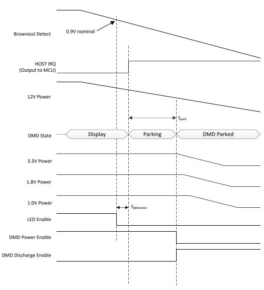
Figure 4. Power-down Timing Diagram
