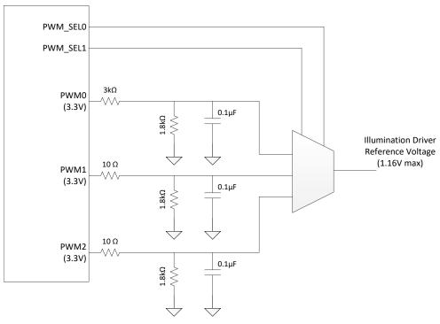
Figure 5. Typical PWM Circuit
