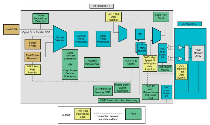
Figure 3. DLP5530S-Q1 Video Path With Diagnostics
