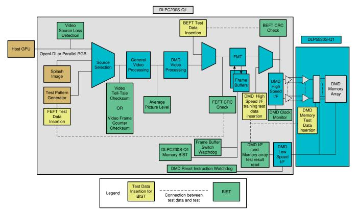
Figure 5. DLP5530S-Q1 Video Path with Diagnostics
