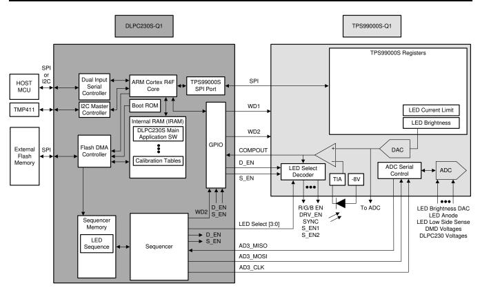
Figure 10. Illumination Control Architecture
