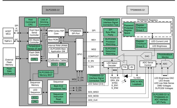
Figure 13. Illumination Control Architecture with Diagnostics
