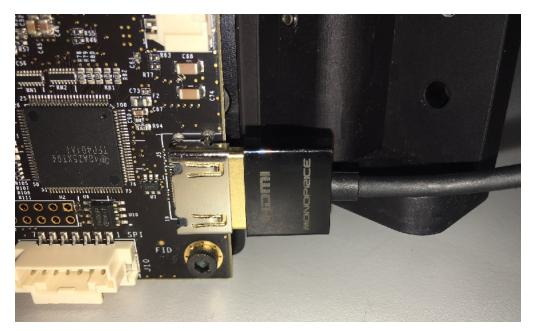
Figure 2-4. HDMI Cable Install
