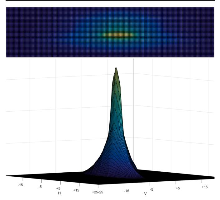
Figure 14. Typical high beam profile
