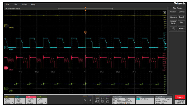
图 3-17. V_{in} = 264\text{Vac} , V_{out} = 20\text{V}
