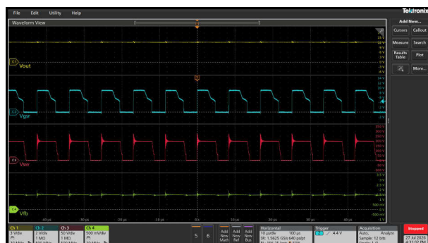
图 3-22. V_{in} = 90\text{Vac} , V_{out} = 12\text{V}
