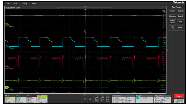
图 3-29. V_{in} = 264\text{Vac} , V_{out} = 9\text{V}
