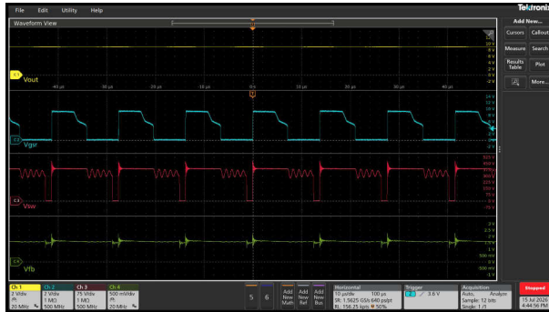
图 3-28. V_{in} = 230\text{Vac} , V_{out} = 9\text{V}
