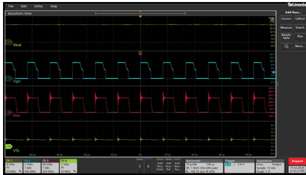
图 3-14. V_{in} = 90\text{Vac} , V_{out} = 20\text{V}
