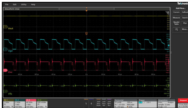
图 3-30. V_{in} = 90\text{Vac} , V_{out} = 5\text{V}
