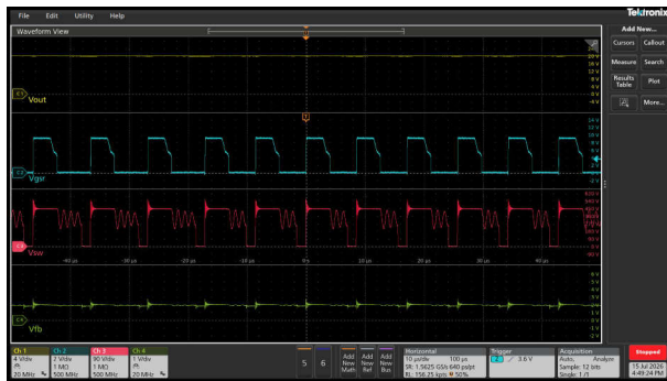
图 3-16. V_{in} = 230\text{Vac} , V_{out} = 20\text{V}
