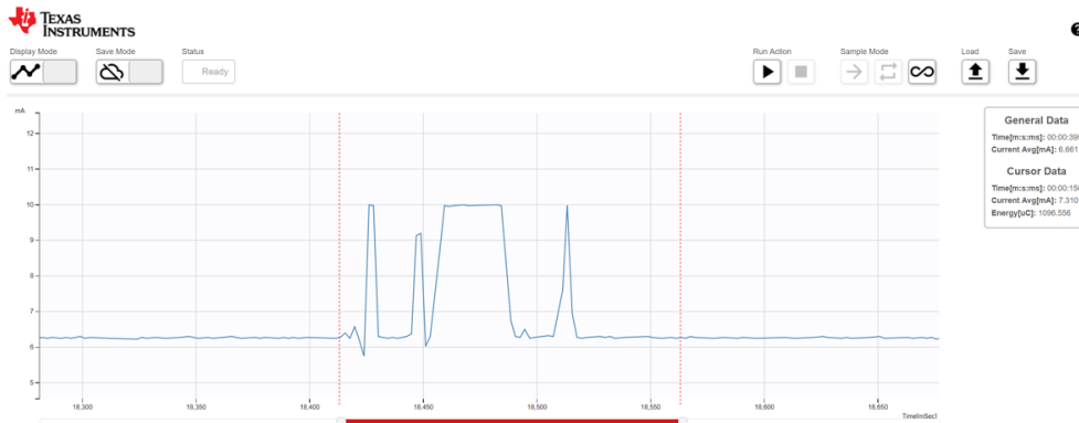
图 31. Collector Current Consumption for Transmission of 150-Byte Data
