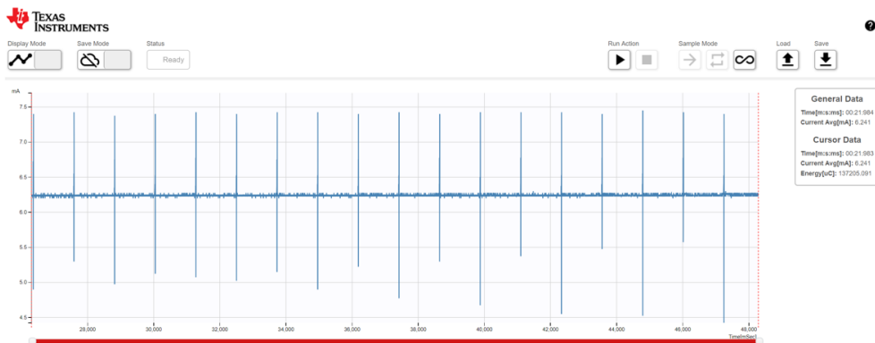
图 26. Collector Current Consumption for 0-dBm Transmit Power
