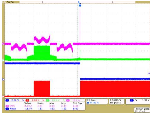
Ch1 – Comparater output (CAOUT) Ch2 – High-side PWM signal input to DRV8305 Ch3 – Motor winding voltage referred to DC minus Ch4 – Motor winding current
