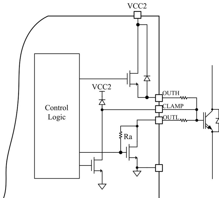
图 7-12. CLAMP, OUTH, and OUTL Clamping Circuits
