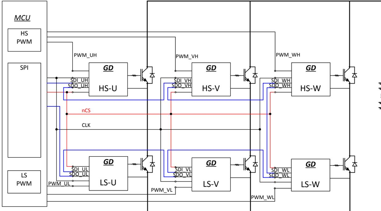
图 7-40. System configuration of daisy chain SPI configuration
