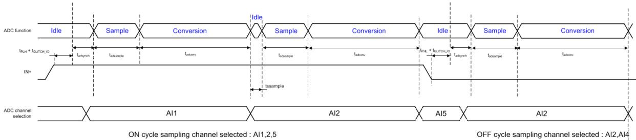
图 7-7. ADC Edge sampling mode timing chart
