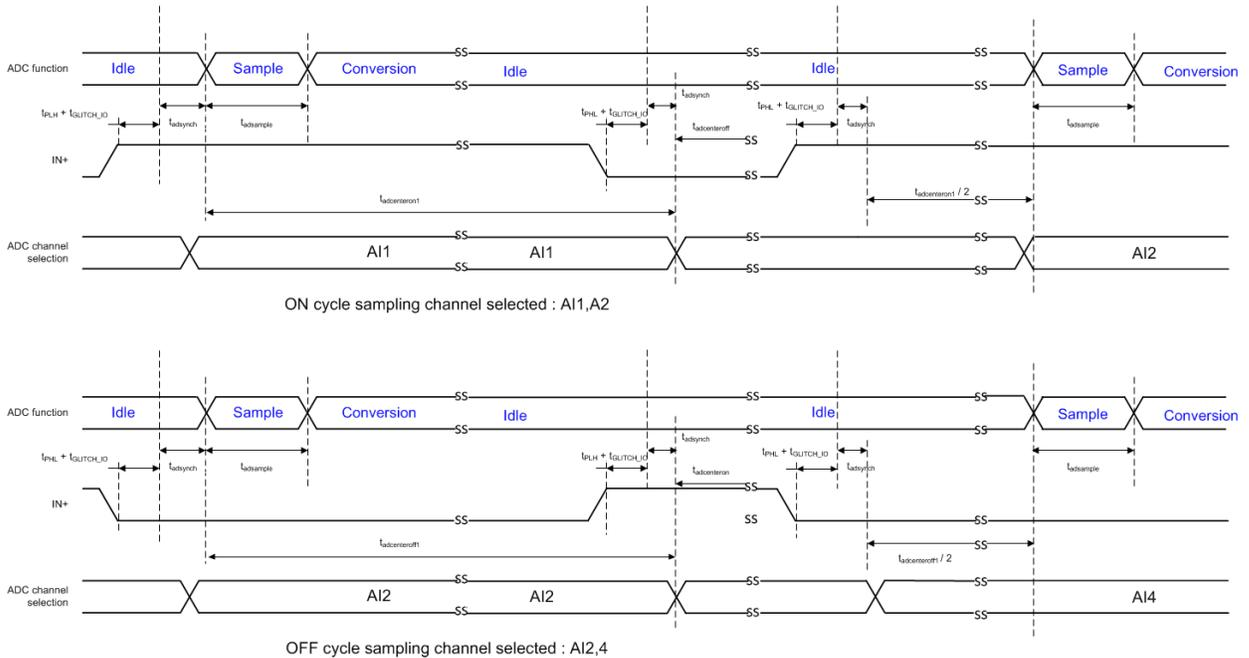
图 7-5. ADC center sample mode timing chart
