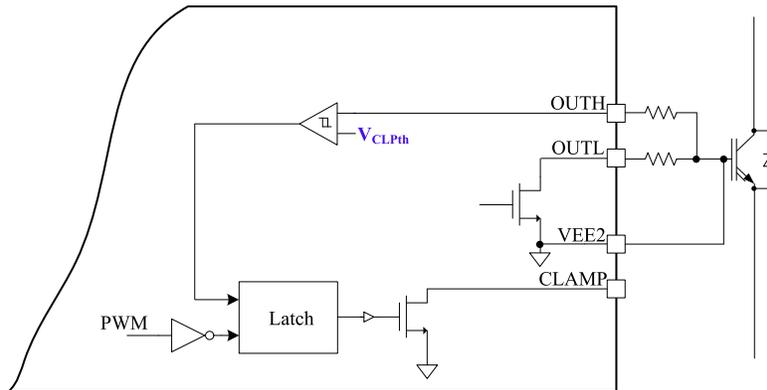
图 7-13. Block diagram of implementation of internal Miller clamp function.
