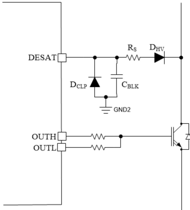
图 8-8. External Components for DESAT
