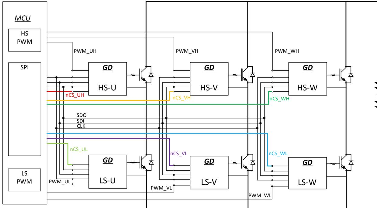
图 7-38. System configuration of regular SPI configuration
