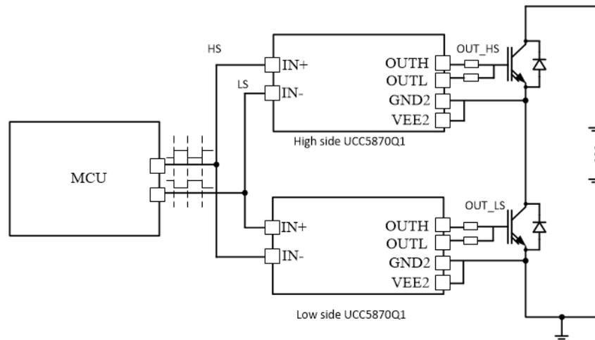
图 7-29. Block diagram of implementation of STP function.
