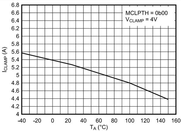
图 6-3. Internal Miller Clamp Current vs. Temperature
