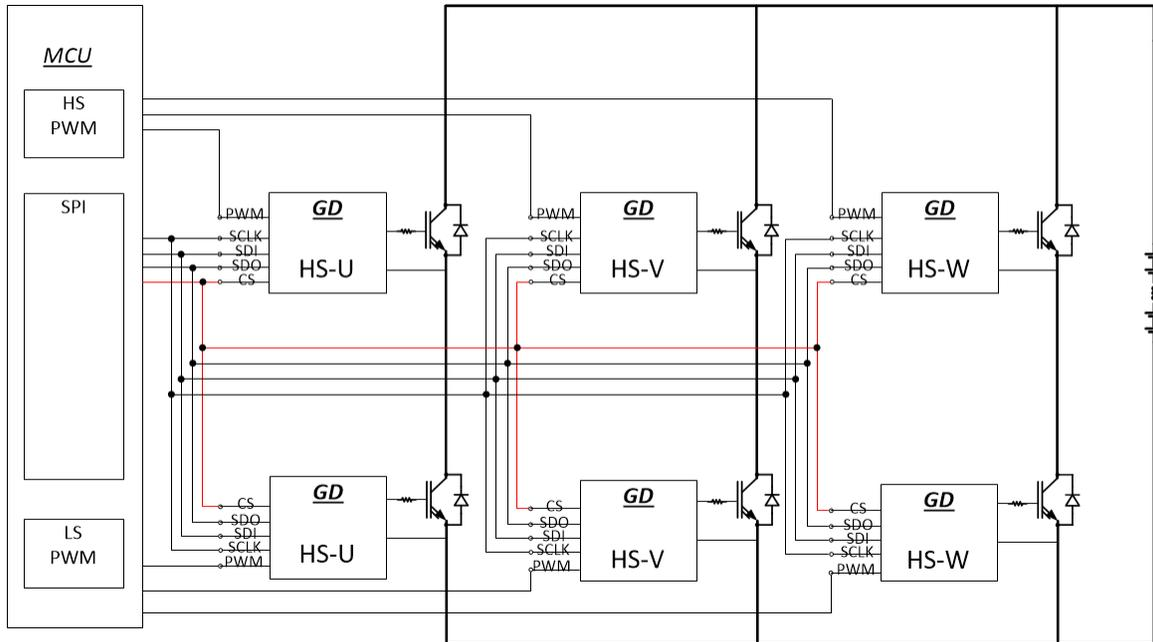
图 7-42. System configuration for Address-based SPI Communication Scheme
