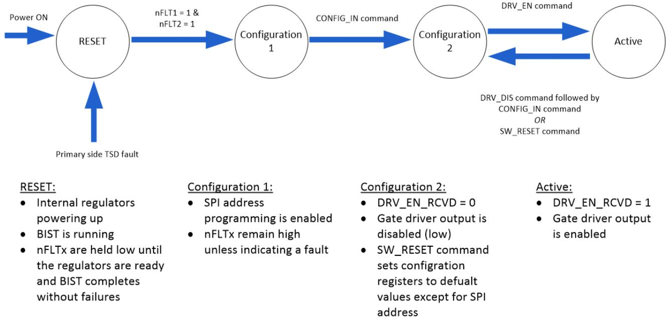
**图 7-37. Operation mode diagram during normal operation**
