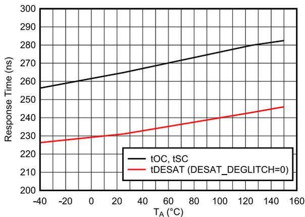
图 6-17. Overcurrent Protection Response Time vs. Temperature
