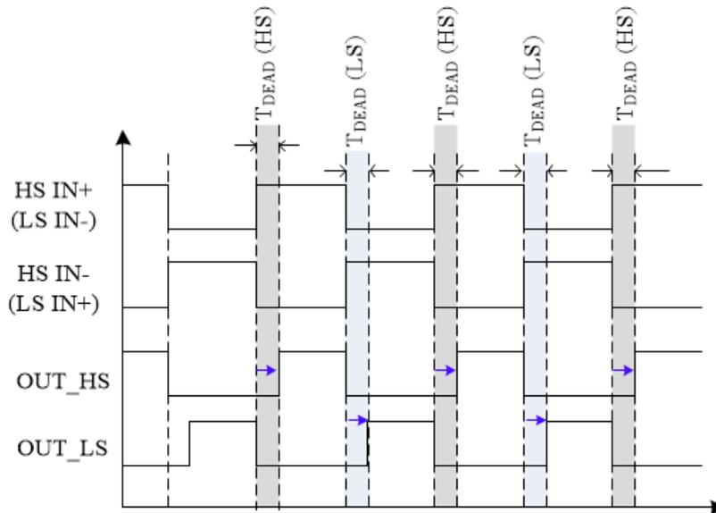
图 7-30. Timing scheme of implementation of STP function.
