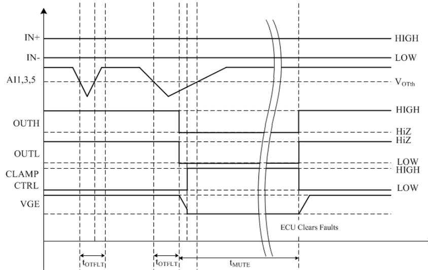
图 7-21. Timing scheme of implementation of PS\_TSD function.
