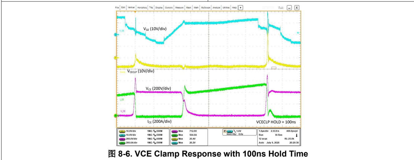
图 8-6. VCE Clamp Response with 100ns Hold Time
