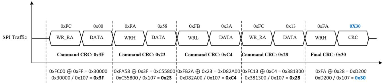
图 7-36. Calculating CRC for a Set of Commands
