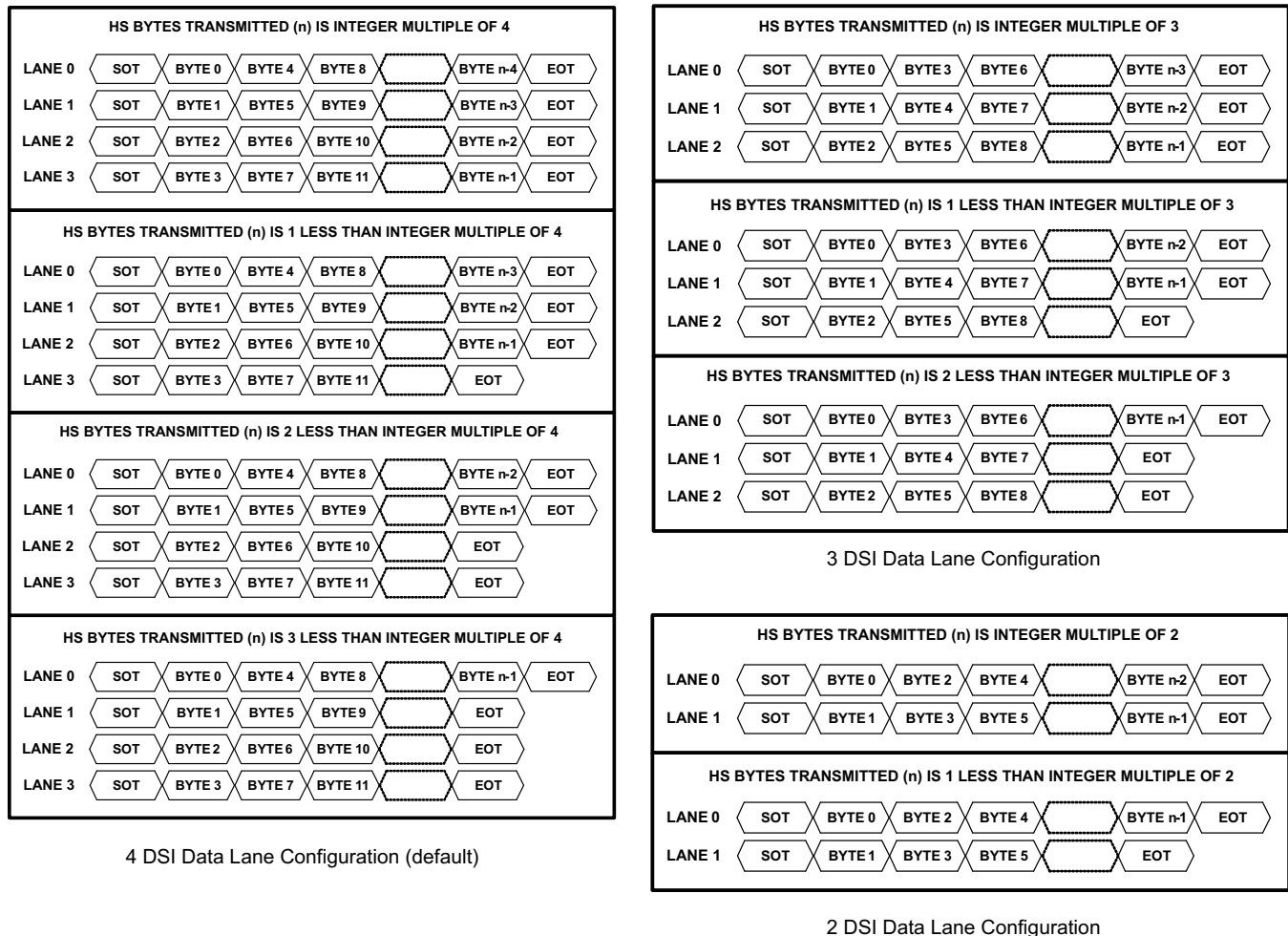
Figure 13. SN65DSI85-Q1 DSI Lane Merging Illustration
