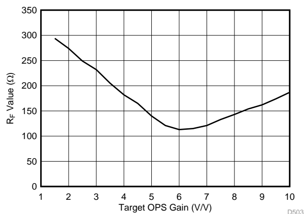
Figure 83. Suggested External R_F Value vs Noninverting Gain for the OPS
