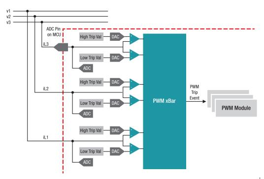
Figure 5. Over current protection scheme on Vienna rectifier
