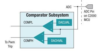
Figure 6. The CMPSS used for overcurrent protection.
