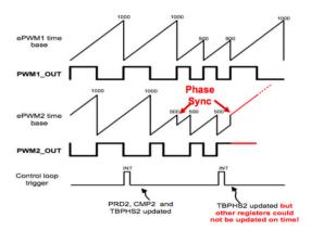
Figure 11. Challenges for variable-frequency PWM waveform generation.
