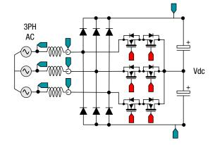
**Figure 2**. Vienna rectifier (Y-connection) topology for EV charging stations.
