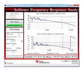
Figure 10. The SFRA run on a closed current loop.
