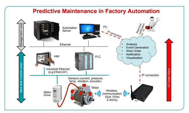
Figure 1. Predictive maintenance in factory automation.
